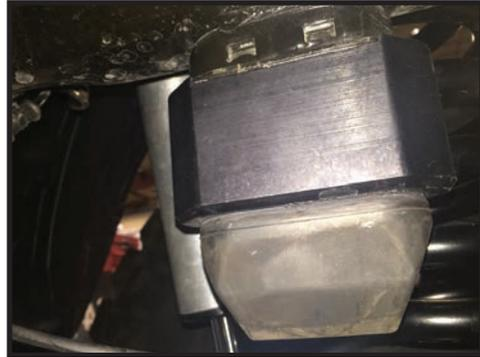
**38.** Install the sway bar drop brackets (214015 & 214016) to the chassis using the factory hardware and tighten using a 15mm socket/wrench. The open side goes toward the center of the truck. [Torque to factory spec] [FIGURE 17]
