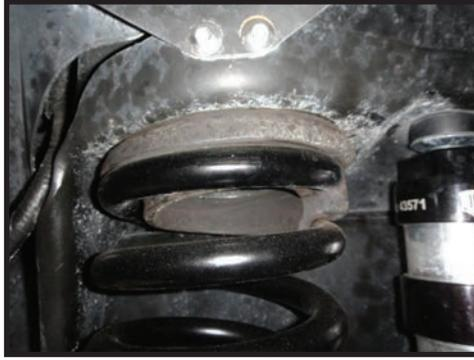
**28.** Slowly raise the axle just before the springs start to compress. Make sure the springs are properly seated before compressing them.
