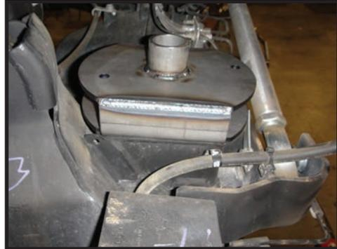
**52.** Set the coil spacers (214105) on the lower coil seats. Bolt them to the seats using the existing holes with the supplied 7/16" hardware. Tighten using a 5/8" socket/wrench. [Torque to 50 ft-lbs] **[FIGURE 19]**
