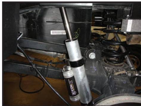
**56.** Remove the rear bump stops from the frame using a 16mm socket/wrench.
