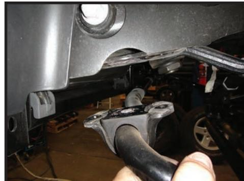
3. Remove the sway bar from the frame using a 15mm socket/wrench. Mark the passenger side of the sway bar and take note to prevent the sway bar from being accidentally flipped during reinstallation. [FIGURE 2]
