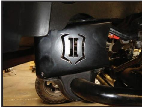
**39.** Mount the sway bar to the drop bracket using the supplied 7/16" hardware with a 5/8" socket/wrench. [Torque to 50 ft-lbs]
