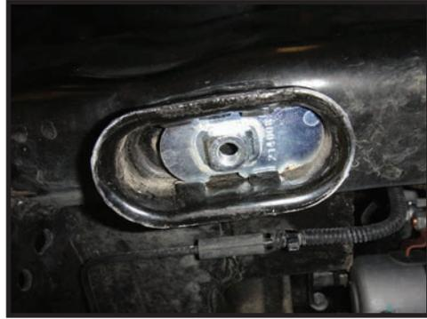
**37.** Mount the bumpstop spacer (217124) to the frame threading it into the retainer plate using the supplied 3/8" hardware, tighten using a 9/16" socket/wrench. [Torque to 30 ft-lbs] Lightly grease and press the bumpstop into the pocket. [FIGURE 15 AND 16]
