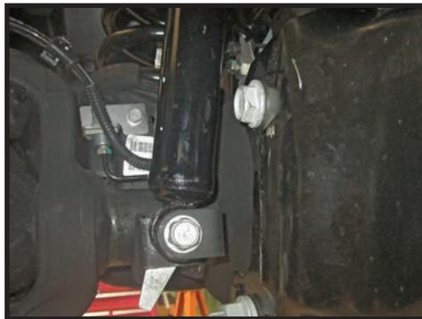
**7.** Slowly lower the jack until the coil springs become loose enough to slide out. Be careful not to damage any brake lines, ABS wires or differential locker wires (Power Wagon only).
