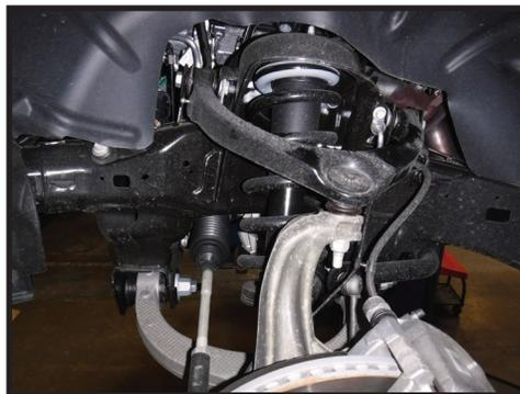
**3.** Starting on the driver side loosen the taper on the upper ball joint using an 21mm socket/wrench. Use a hammer to separate the upper ball joint taper and tie rod end. Support the spindle so that it does not over extend the CV joints when detached. [FIGURE 2]
