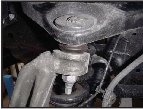
**4.** Using a 18mm wrench remove the two bolts securing the UCA to the vehicle. [FIGURE 3]
