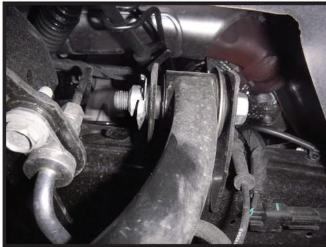
**5.** Install your new ICON driver billet UCA in to the UCA frame pockets using factory hardware making sure the heim spacers (157432) are installed in the rod end and torque to factory specs. [FIGURE 4 & 5]
