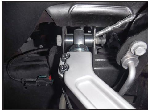
**6.** Install the ball joint into the spindle and tighten using the supplied nut and 18mm socket/wrench. [Torque to 75ft-lbs] [FIGURE 6]
