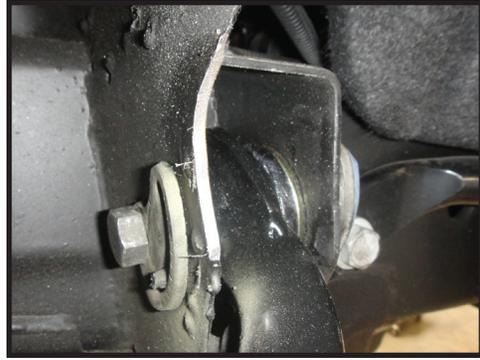
**8.** With the control arm completely assembled, slide the arm into the upper mounts (with large washers on each side of the bushings) and insert the OEM hardware loosely.
