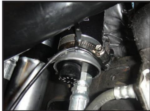
9. Install the supplied (174037) stem top adapter on top of the shock bucket, taking care to note that the middle hole is offset to bring the shock outward for clearance. Using the supplied 9/16" hardware, fasten the adapter mount using a 13/16" wrench and 7/8" socket. [FIGURE 6 & 7]
