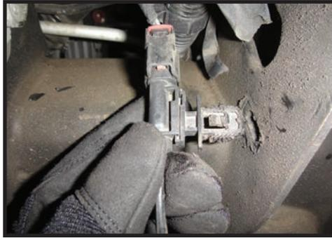
7. The supplied (250002) reservoir bracket will be installed into the large hole where the ABS clip was removed. Use the supplied (150014) nut tab and 3/8" bolt to fasten the reservoir bracket to the bucket as shown. [Torque to 45 ft-lbs] [FIGURE 2 & 3]
