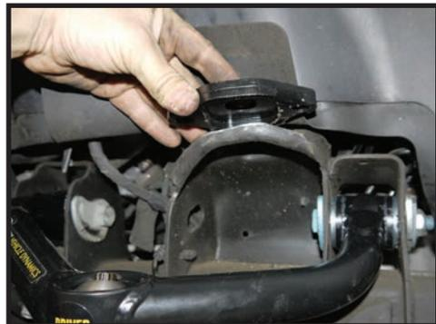
10. Slide the shock into the shock mount making sure to have the bushings on prior to final installation.
