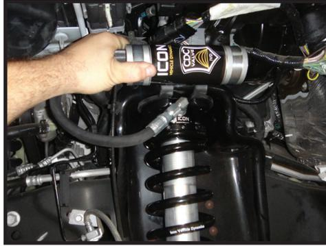
NOTE: failure to use the supplied reservoir bracket will cause the hose fitting to crash into the coil bucket.
