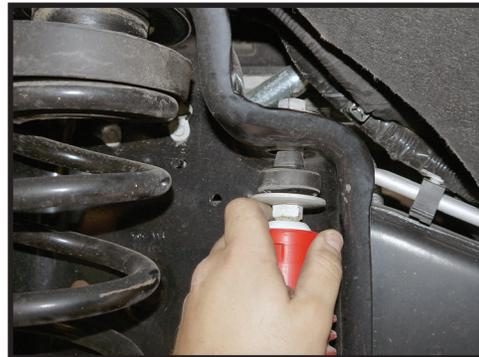
**3. Remove trackbar bolt at frame. [FIGURE 3]**
