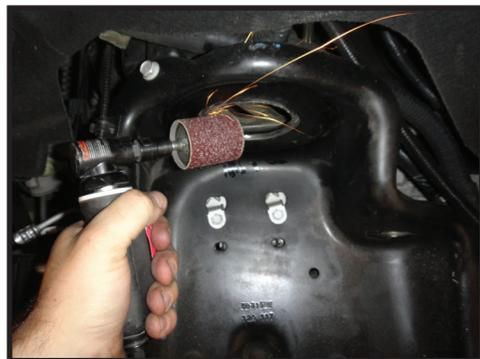
**8. Sand any material that keeps the upper coil bucket from being flat. [FIGURE 9]**
