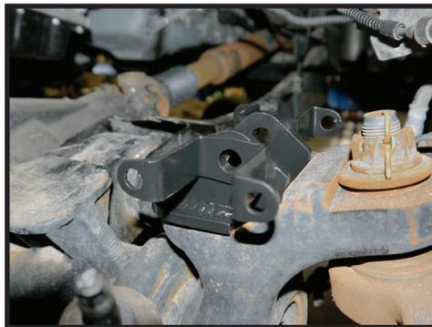
**14.** Using the supplied 5/16" hardware, install the factory lines that were attached to the factory lower coil seat with a 1/2" socket/wrench. [Torque to 24 ft-lbs]
