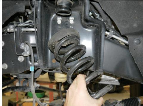
**5. Remove the lower coil mount with a 22mm socket/wrench and the lines attached to it using 10mm socket/wrench. [FIGURE 6 & 7]**
