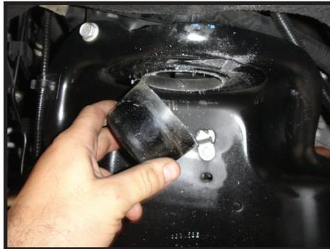
8. Grind any material that keeps the upper coil bucket from being smooth and flat. [FIGURE 9]
