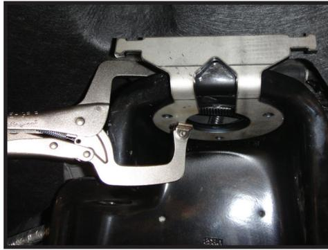
**10.** Using a transfer punch, mark the locations of all 3 holes in the reservoir bracket.
