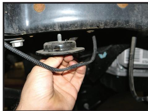
**16.** Install the driver side coilover: The reservoir hose will point towards the front of the vehicle indicating the driver side. With the reservoir bracket sandwiched between the coil bucket and the coilover mount, use the supplied 3/8" hardware to fasten the coilover to the coil bucket. [Torque to 45 ft-lbs] Twist the hose and loop around to the reservoir mount as shown. Attach the reservoir to the mount using the supplied hose clamps with a 5/16" socket/wrench. [FIGURE 14]
