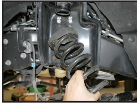
5. Remove lower coil mount with a 22mm socket/wrench and the lines attached to it using 10mm socket/wrench. [FIGURE 6 & 7]
