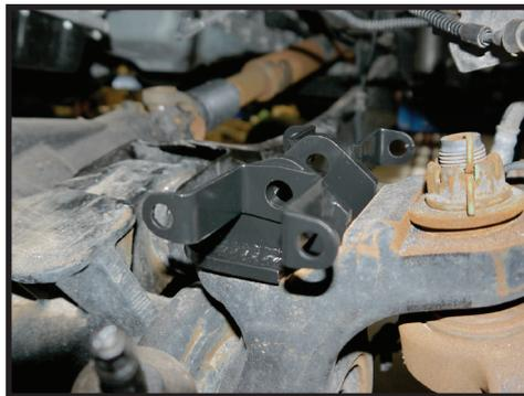
**14.** Using the supplied 5/16" hardware, reattach the factory lines that were attached to the factory lower coil seat with a 1/2" socket/wrench. [Torque to 24 ft-lbs]
