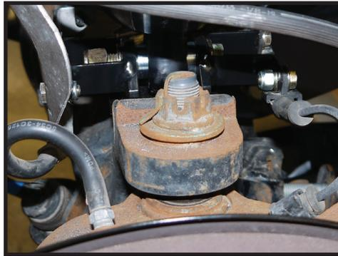
**21.** Install new alignment cam supplied in kit: make sure arrow is pointing toward front of truck and flat end of cam is aligned with flat end on knuckle. Use the old cam to tap in the new cam and install castle nut. [Torque to 69 ft-lbs] Install cotter pin.
