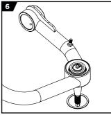
STEP 6: Install retaining ring & reinstall grease fitting. Take care not to overtighten zerk.
