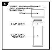
STEP 4: Arrange Delta Joint, UCA, and adapter tube as shown. If installing in an ICON billet UCA that has an angled bore, the tapered shim (\*shown in diagram) is required. This shim is available in ICON Part #614520 and #614518.
