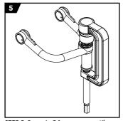
STEP 5: Screw in C frame screw until Delta Joint is seated. Failure to use tapered shim on ICON UCA with angled bore will destroy the bearing bore.
