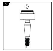
STEP 3: Remove grease fitting from Delta Joint. Failure to remove may lead to terminal damage if press used doesn't allow clearance for zerk to pass through.
