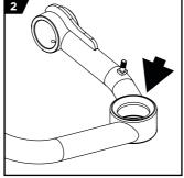
STEP 2: Clean UCA bore & retaining ring groove. Once clean, liberally apply antiseize to bore.
