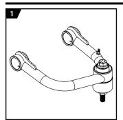
STEP 1: Remove retaining ring and press uniball out of UCA. If using ICON Uniball Replacement Tool Kit see Part #614518 instructions.
