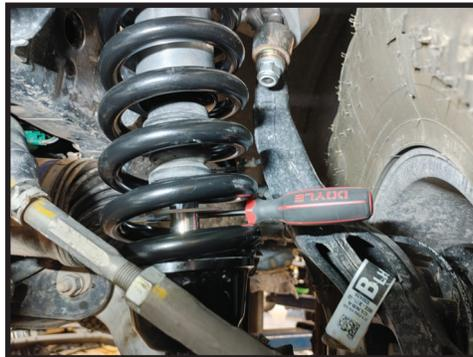
2. Next, slip the spacers between the coils and let them fall into the coil cup. [FIGURE 2]
