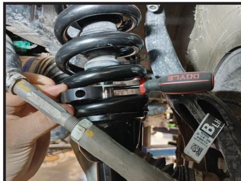
3. Position the spacers so that you can thread the supplied 10-24 x 1.000 SHCS into the spacers using a 5/32 hex key. [FIGURE 3 & 4]
