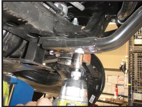
**5. (NON KDSS VEHICLES ONLY)** Disconnect the sway bar from the frame on both sides. Remove bolts using a 14mm socket/wrench and remove the bracket from the sway bar. Move the sway bar forward to make room for removal and installation of the shock.
