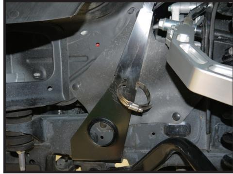
**16. (KDSS ONLY)** On KDSS equipped vehicles there is a tab located on the driver side frame rail of the vehicle. This tab will need to be cut off to allow for installation of the shock reservoir bracket (154005). [FIGURE 7]
