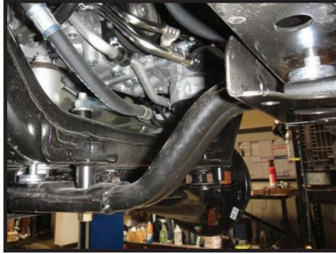
**23.** Slightly bend the hanger tabs down on the factory skid plate, they will no longer be used. [FIGURE 11]
