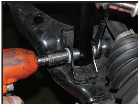
**12.** If replacing the upper control arms, refer to appropriate UCA instructions now. Mount the upper control arm to the knuckle and tighten the taper nut. [Torque to factory spec]
