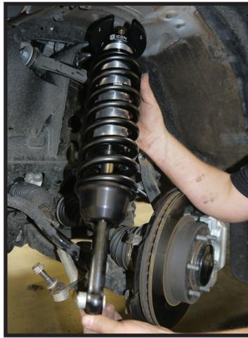
**9.** Connect the shock to the lower control arm: The lower shock mount has (1) long and (1) short spacer [Torque to factory spec]. Make sure the long spacer is toward the front of the vehicle as this will position the shock further toward the rear of the control arm to ensure adequate sway bar clearance. Install the factory lower shock bolt.
