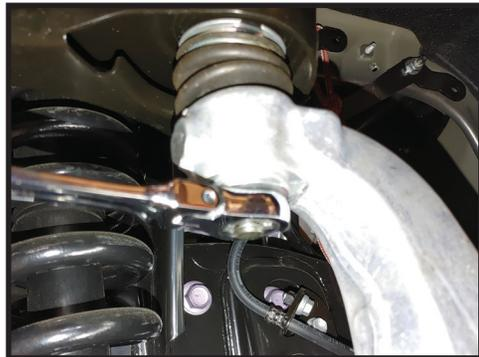
**14.** Use a hammer or balljoint separator to loosen the balljoint taper from the spindle. [FIGURE 14]
