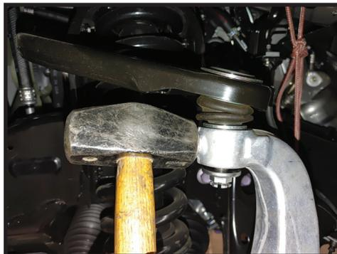
**15.** Loosen and remove the UCA pivot bolt from the frame using a 22mm. [FIGURE 15]
