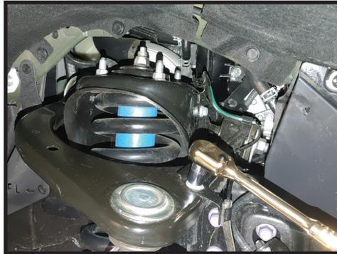
**13.** Remove the cotter pin from the UCA balljoint using a small screwdriver or pick to pry over the safety clip, and pull out the pin using a needle nose pliers. Loosen the 19mm nut on the balljoint. [FIGURE 12 & 13]
