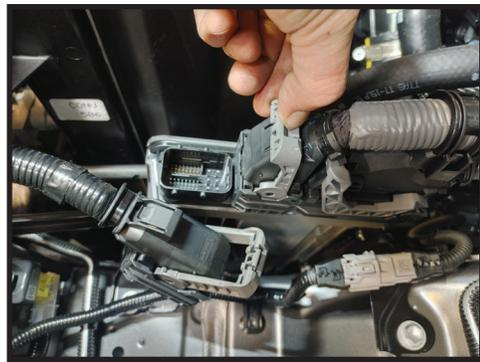
9. Remove the harness clamp from the large wire loom using a small flat blade screwdriver. [FIGURE 7]
