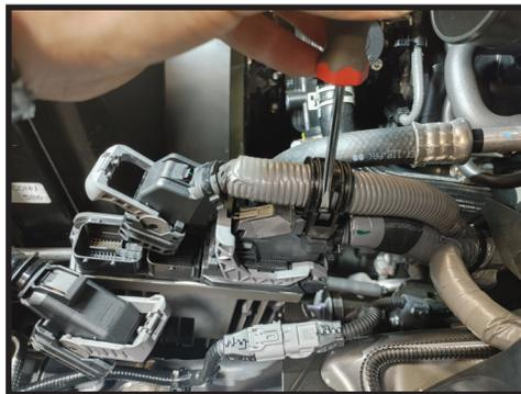
10. Remove the large harness from the ECU. Press lock clip and pull up on the grey lever and pulling plug out. [FIGURE 8]
