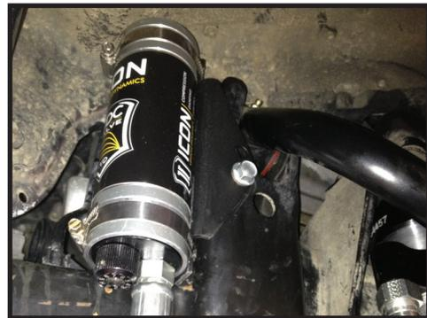
**12.** Rotate the reservoir and bracket so that the reservoir is just over the top of the frame rail and tighten both the clamps and the bracket mount bolt.
