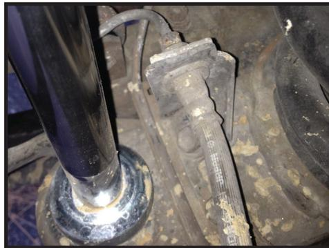
**13.** Check component clearances at full droop. Sway bar drops and/or extended break lines may be necessary with the additional down travel.
