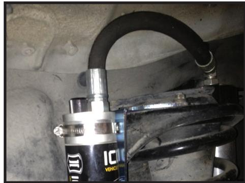
**12.** Some vehicles have a brake line bracket near the bottom mounting of the shock that can interfere with the shock body on full compression. It may be necessary to bend the bracket away from the shock slightly. [FIGURE 4]
