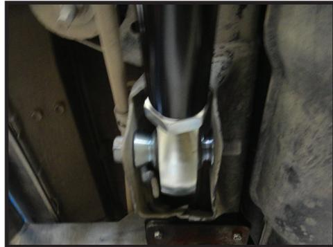
**7.** Tighten jam nut using an 1.5" open end wrench. [Torque to 200 ft-lbs] Make sure the rod end is vertical as it is tightened.
