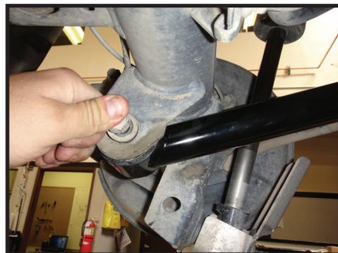
**5.** The pinion angle can be adjusted as desired once both links are installed. Do not adjust longer than 3.5". [FIGURE 3]
