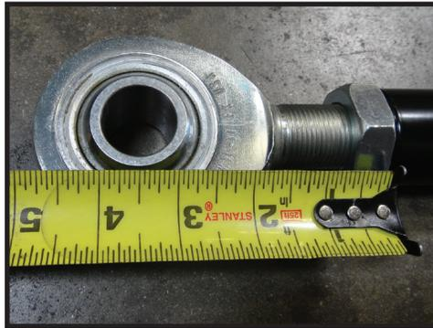
**6.** Connect the link to the frame using the factory hardware with the short spacer towards the inside of the vehicle. This will move the front link pivot points closer together on the frame to help correct roll-steer geometry on lifted vehicles. [FIGURE 4 & 5]
