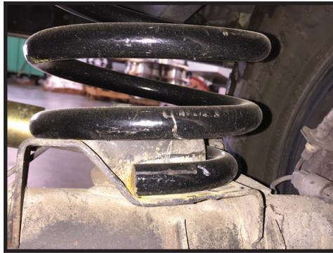
**7.** Use a jack to raise the axle, compressing the springs a couple of inches but NOT to the point where it lifts the vehicle off the jack stands.
