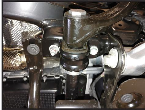
5. Support the lower control arm and remove the bolts from the frame. Remove the 15mm nuts from the top of the coilover. [FIGURE 4]
