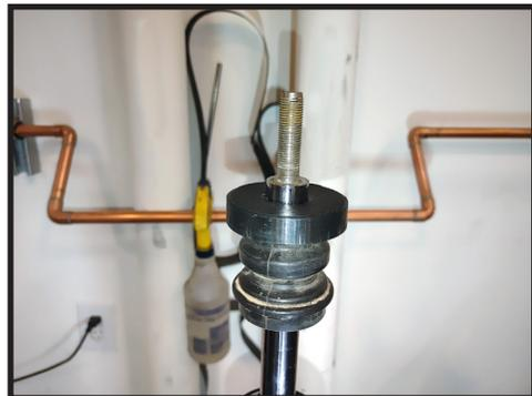
**11.** Install the factory coil spring onto the body in the same direction as factory. The tag/mark on the coil should be facing the frame when installed on the truck. Make sure the spring is sitting correctly on the spring isolator. The front of the Icon EXP can be determined by the lower barpin, the short end faces the front, the longer end faces the rear. [FIGURE 14]
