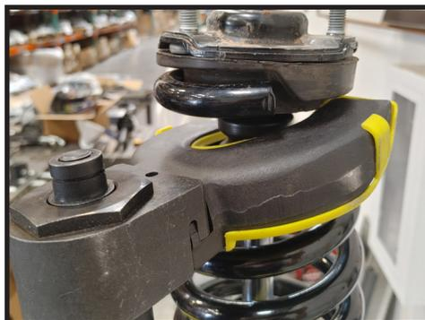
**15.** Install and tighten the 1/2-20 flanged nylock nut to 40 ft-lbs. An 8mm wrench can be used to keep the shaft from spinning.
