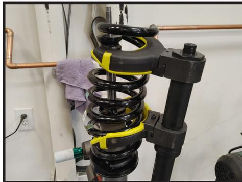
**14.** Install the upper mount onto the shaft and make sure the orientation is correct and the same as factory. Also be sure the isolator is positioned correctly with the spring. [FIGURE 17]
