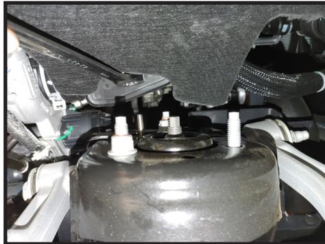
6. Remove the 18mm nuts from the bottom of the coilover. [FIGURE 5]
