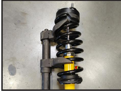
**9.** Set the factory coilover aside. Grab the new Icon EXP coilover and install the spring perch snap ring, spring perch and spring isolator. Refer to page 7 for the groove options for your particular Bronco and trim level. [FIGURE 8, 9, 10, 11]
