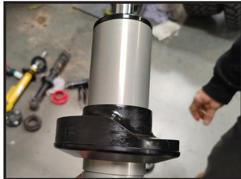
**10.** If running 37" tires tall tires, remove the spacer on top of the foam bump stop and install part# 611082. [FIGURE 12 & 13]
