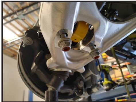
7. Remove the lower control arm pivot bolts using a 24 and 21mm. Lower the arm down so the coilover can be removed. Mark the coil if the tag has been removed. The tag/mark should be facing the frame. You may need to pry on the arm/coilover to get the lower studs out of the arm [FIGURE 6]
