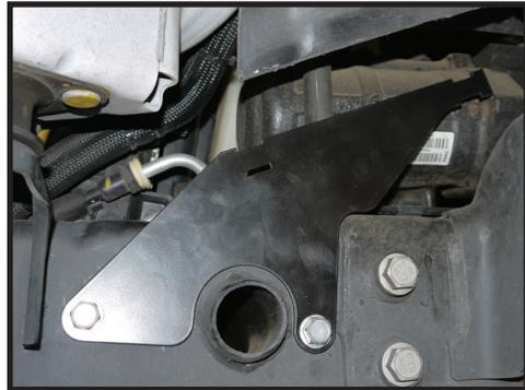
**12.** Inspect the opposite side of the frame rail, checking for any hoses or lines that have to be temporarily removed or held out of the way. Center punch and drill to 21/64”.
