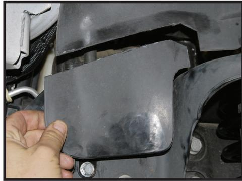
**11.** Orient the reservoir mounting bracket on frame rail forward of the coil bucket and mark center of the 2 holes. [FIGURE 7]
