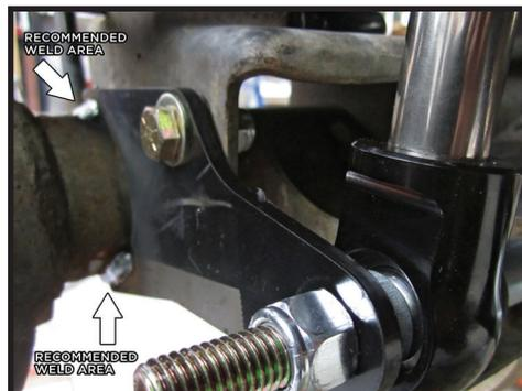
**5.** Line up the doubler plate eyelet and the OEM shock mount by sliding the supplied 1/2" X 4.5" bolt through the doubler plate and the OEM shock mount. Tighten the 3/8" locator bolt to secure the doubler plate in position.
