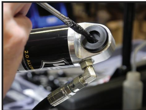
**6.** You will need to lightly chamfer the bar pin to allow it to slide in to the bushing easily. Slide the bar pin (chamfered end first) into the greased eyelet bushing as far as you can by hand, it will not be fully seated but it will be held in place until you press it in to the bushing. [FIGURE 2]
