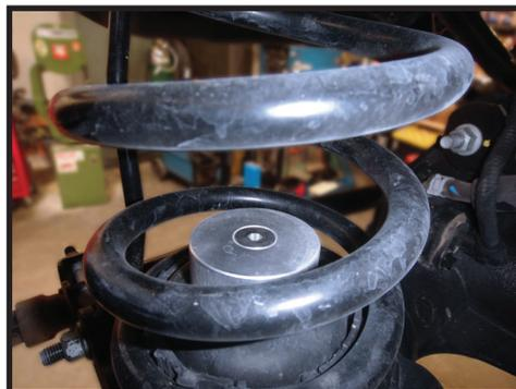
3. On the passenger side, remove the brake line bracket from the back of the coil seat using a 10mm. This allows easier access under the striker pad.
