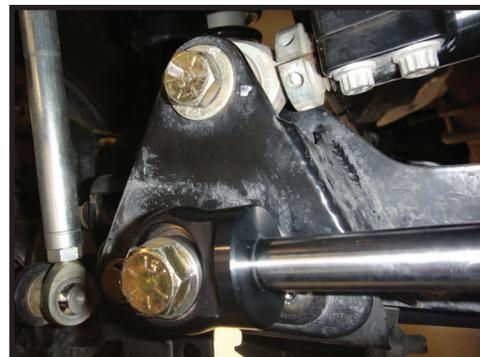
7. Check to make sure the wheels are still straight. **VERY IMPORTANT!** Using the supplied shock shaft spacer, slide the shock body until the shaft spacer hits the aluminum cap on the end of the shaft and the seal head of the shock body. This centers the stabilizer in its travel. Turning the 'Drive Zone' adjuster counter clockwise will soften the shock and make it easier to move. [FIGURE 3]
