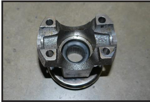
**7.** Slide the new yoke onto splines of the output shaft of the transfer case. Using the stock nut and thread lock [Torque to factory spec] (FIG. 6).
