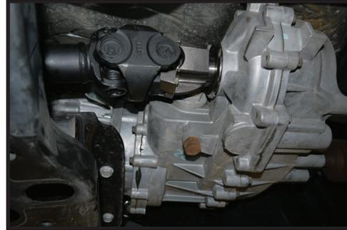
**8.** Connect the driveshaft to the transfercase yoke using the supplied 5/16" hardware. Use a 5/16" 12-pt or a 1/2" 6-pt depending on the supplied hardware. Use a small amount thread lock on the threads of the bolts [Torque to 21ft-lbs] (FIG.7).
