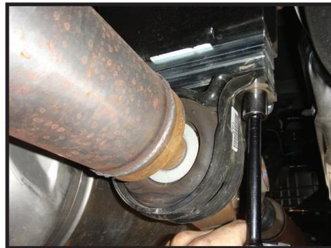
2. Install (217127) carrier bearing drop bracket with supplied hardware using a 17mm socket/wrench. [Torque to 45 ft-lbs]
