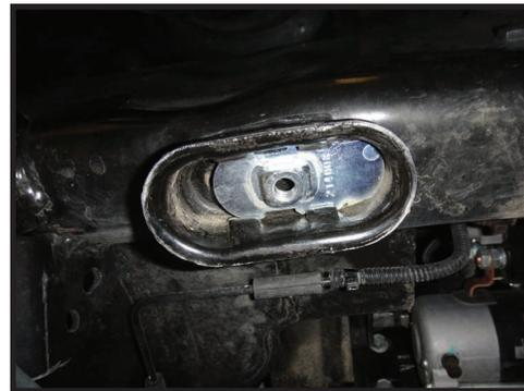
4. Mount the bumpstop spacer (217124) to the frame threading it into the retainer plate using the supplied 3/8" hardware, tighten using a 9/16" socket/wrench. [Torque to 30 ft-lbs] Lightly grease and press the bumpstop into the pocket. [FIGURE 3 AND 4]
