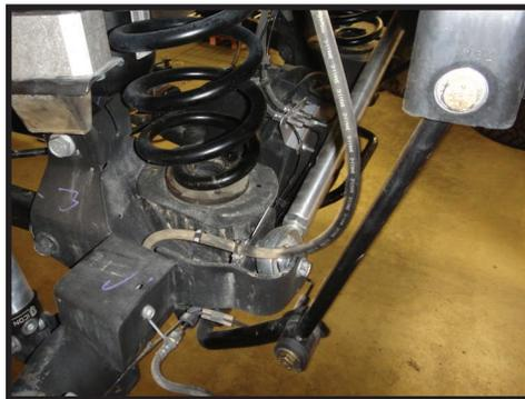
4. Check the torque on all hardware. Drive the truck 1-2 miles and re-torque all nuts and bolts.
