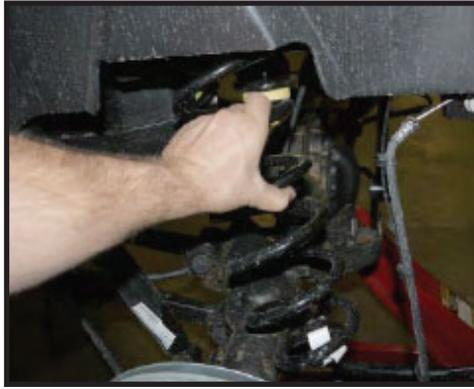
5. Install the ICON coils and lift the axle enough to connect the shocks. Connect the shocks using (2) 21mm. [FIGURE 4] [Torque to factory spec]
