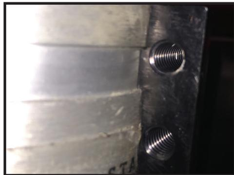
**9.** Make sure that the inner locking portion of the collar is securely seated inside the groove on the shock body. As you release tension make sure you have maintained alignment with your marks. By putting a rod or extension in the lower eyelet you can visually check that it is in line with the 3rd mount bolt. [FIGURE 15]
