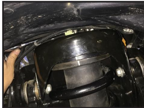
**3.** Disconnect the tie rod and upper arm from the knuckle: Loosen the nuts using an 18mm and 21mm and strike the side of the knuckle at the taper to dislodge. Support the top of the knuckle to prevent it from flopping outward and over extending the CV joints. Disconnect the sway bar link at the sway bar using an 18mm. [FIGURE 3]
