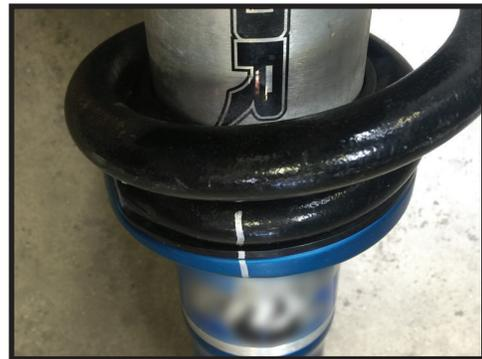
**6.** It is not necessary to disassemble the shock or coil, however the spring will need to be compressed a couple of inches. A quality spring compressor is necessary; we recommend a three arm style as shown in the photos. [FIGURE 8]
