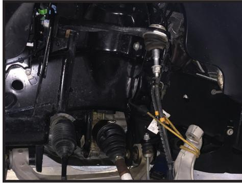
**LIVE VALVE ONLY:** Follow the Live Valve back to the connector then disconnect the Live Valve and wire retainers. [FIGURE 4 & 5]
