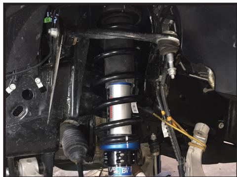
**10.** Reinstall in vehicle: slide the upper 3/8" ring over the three studs. Secure the upper mount with the supplied flange lock nuts and blue thread locker [Torque to 33 ft-lbs]. Reinstall lower shock bolt. Reinstall upper ball joint to knuckle, tie rod, and sway bar link. [Torque to factory spec]
