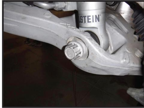
**9.** With the factory coil over removed mark the upper and lower mount on the coilover. This will aid in reassembly and installation of coil over later [FIGURE 9 & 10]
