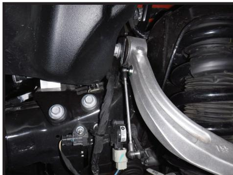
**8.** Using a 16 mm wrench remove the top three nuts that secure the coilover in place. Once completed remove the lower coilover bolt using a 30mm sock/wrench. The coil over can be completely removed at this point. [FIGURE 7 & 8]
