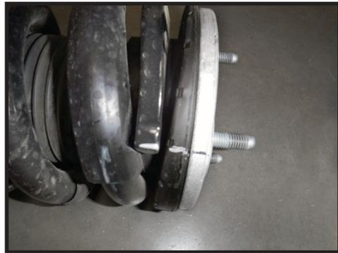
**10.** Compress the spring using a spring compressor and remove the upper coil over mount using a 20mm socket. [FIGURE 11]
