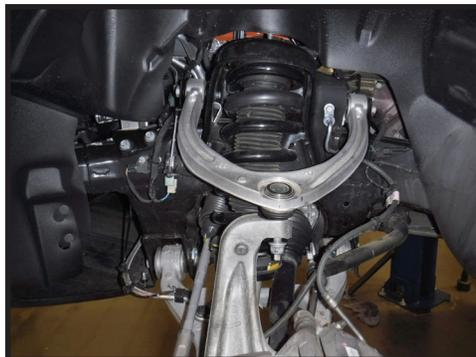
**7.** Using a 10 mm wrench remove the ball off of the side of the control arm [FIGURE 6]
