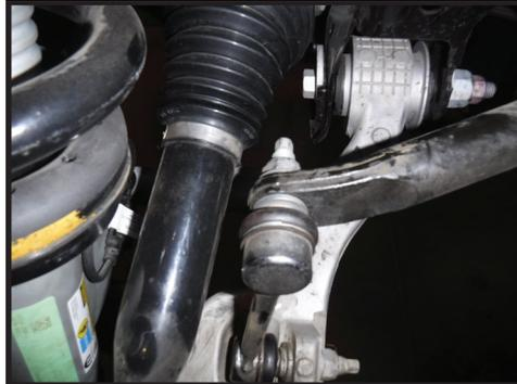
**6.** Loosen the taper on the upper ball joint and the tie rod end using an 21mm socket/wrench. Use a hammer to separate the upper ball joint taper and tie rod end. Take care not to damage the threads. Support the spindle so that it does not over extend the CV joints when detached. [FIGURE 5]
