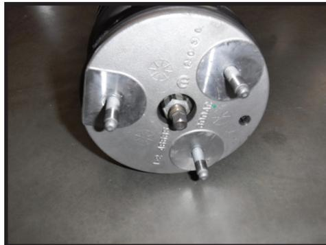
**11.** Remove upper mount from the coilover. Take off the boot and factory rubber isolator. Once the boot is removed knock the three 10mm studs out with a hammer. [FIGURE 12]
