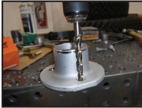
**13.** Once all three holes are drilled install 605234 studs into the top mount using a hammer and punch. Make sure studs are pressed in all the way and are flat against the machined surface. [FIGURE 14]
