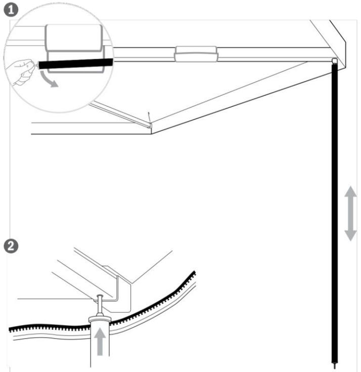
**TIP** IN CASE OF RAIN, LOWER THE SUPPORT LEGS TO ALLOW DOWNWARD SLOPE AND GUY OFF BETWEEN RAFTERS TO FORM VALLEYS FOR WATER RUN-OFF.
